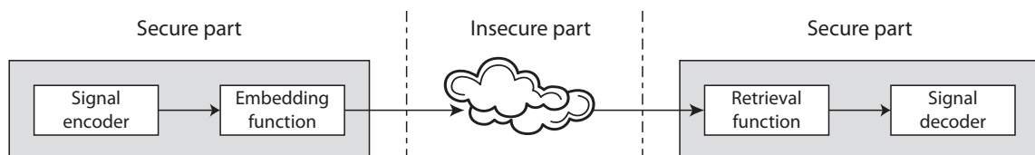
Figure 3.16: Transmission scheme with watermarking.
