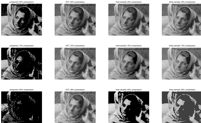
Figure 9.2: Thresholding compression of the image from Figure 9.1 for different dictionaries and compression ratios. The first column shows the component-wise representation, the second column shows the discrete cosine transform (DCT) representation, the third column shows the Haar wavelet representation and the fourth column shows the discrete Meyer (dmey) wavelet representation. The first rows show a truncation giving a 2 : 1 compression (50% of coefficients zero), the second row a 4 : 1 compression (75% of coefficients zero) and the third row a 10 : 1 compression (90% of coefficients zero).
