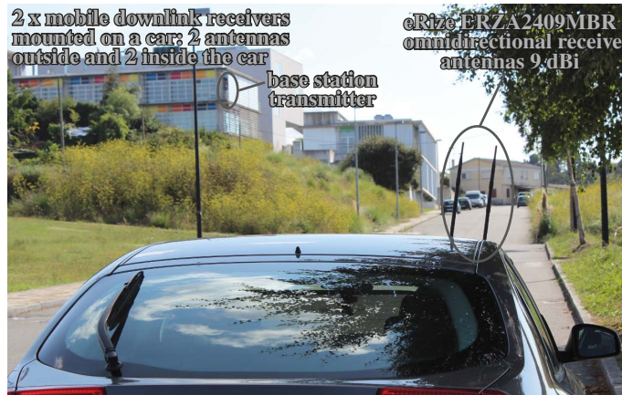
Figure 6.4: Mobile receivers mounted on a car. Two antennas corresponding to the outdoor receiver are placed on the roof of the car, while another two antennas for the second receiver are inside the car, between the two front seats.
