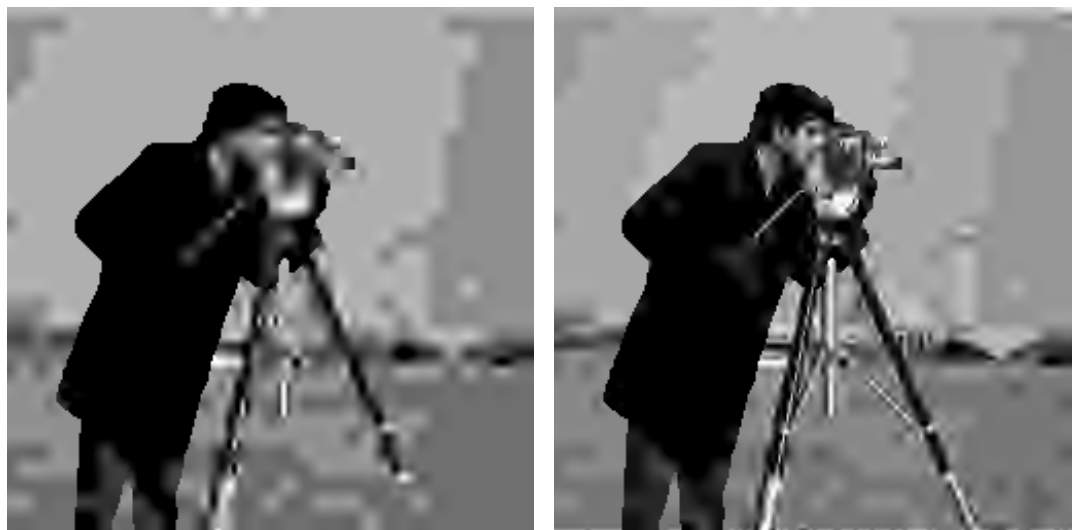
(a) q = 256 , \Delta R = -0.00026 bpp, PSNR = 20.65 dB (b) q = 128 , \Delta R = -0.006 bpp, PSNR = 23.32 dB
