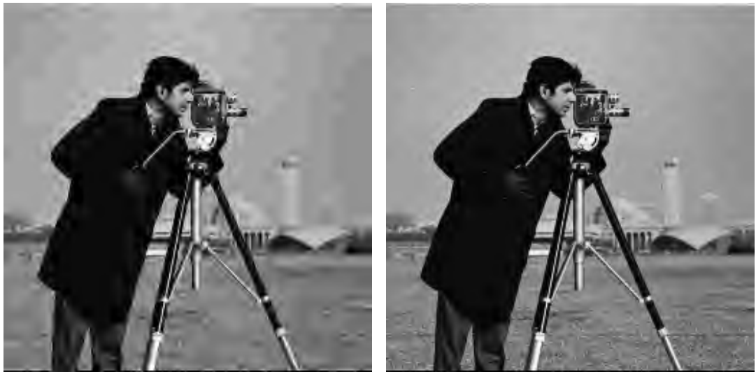
(c) q = 64 , R = 0.30 bpp, PSNR = 26.43 dB (d) q = 32 , R = 0.55 bpp, PSNR = 30.05 dB
