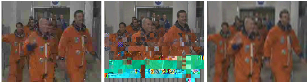
(f) Bad state, EEP, low source bit-rate (g) Bad state, EEP, high source bit-rate (h) Bad state, UEP
