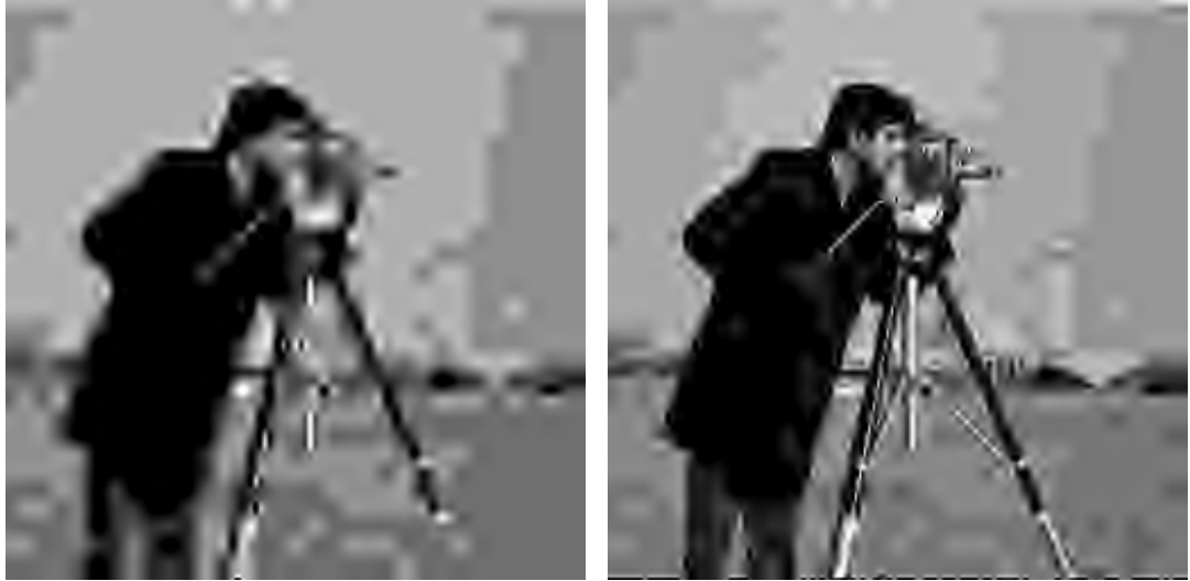
(a) q = 256 , R = 0.08 bpp, PSNR = 20.25 dB (b) q = 128 , R = 0.16 bpp, PSNR = 22.98 dB
