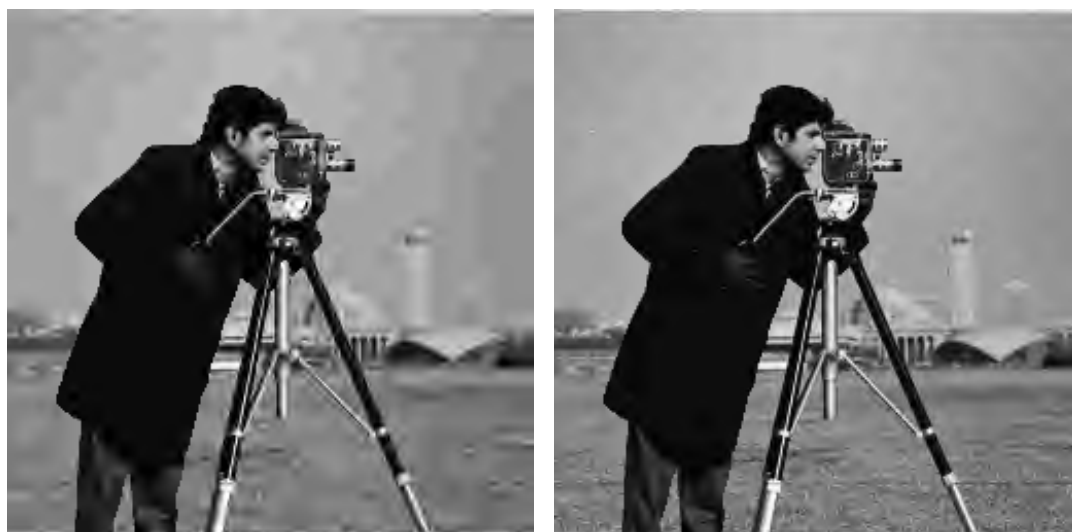
(c) q = 64 , \Delta R = -0.0165 bpp, PSNR = 26.69 dB (d) q = 32 , \Delta R = -0.028 bpp, PSNR = 30.12 dB
