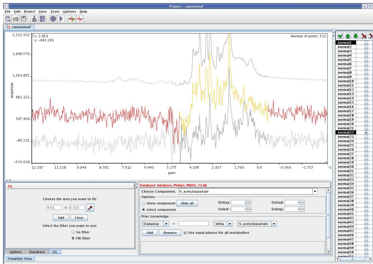
Figure 7.7. Main frame of AQSES GUI. A project with many MRS signals is loaded. The settings of the AQSES quantification method can be modified in the bottom part of the view.
