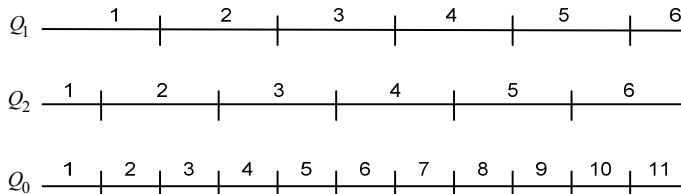
Figure 4.2: An example of a balanced two-description MDSQ with the center of the cell reconstruction.
