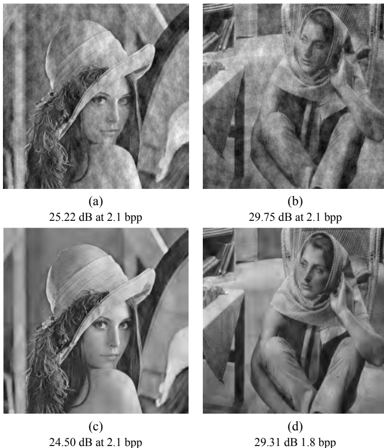
Figure 5.12: Visual comparison of images reconstructed using the central quantizer at level \mathbf{p} = [1, 1] . Images (a) and (b) are the reconstructions using the asymmetric EIA [51]. Reconstructions using the proposed optimized SSMDQ are shown by the images (c) and (d). The reported rate is the sum rate of two sides, i.e., R = R_1 + R_2 .
