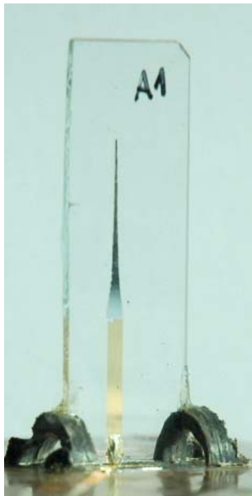
Figure 6.21: The resistively loaded monopole mounted on a ground plane.
