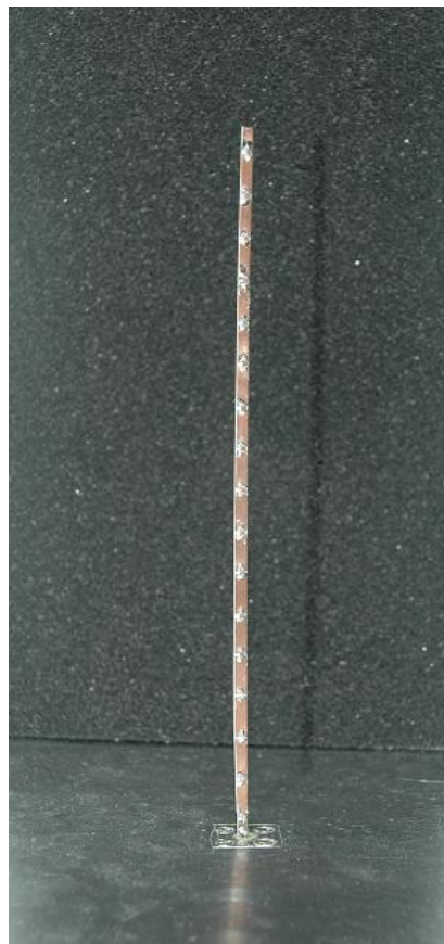
Figure 6.11: Capacitively loaded monopole optimized in the section 5.4, scaled to the frequency band 0.5 GHz-2.1 GHz
