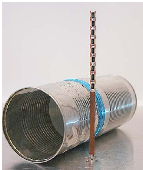
Figure 6.6: Metallic can (diameter=73mm, length=187 mm) used as a Wheeler cap for J-G radiation efficiency measurement of the 150mm long resistively loaded antenna
