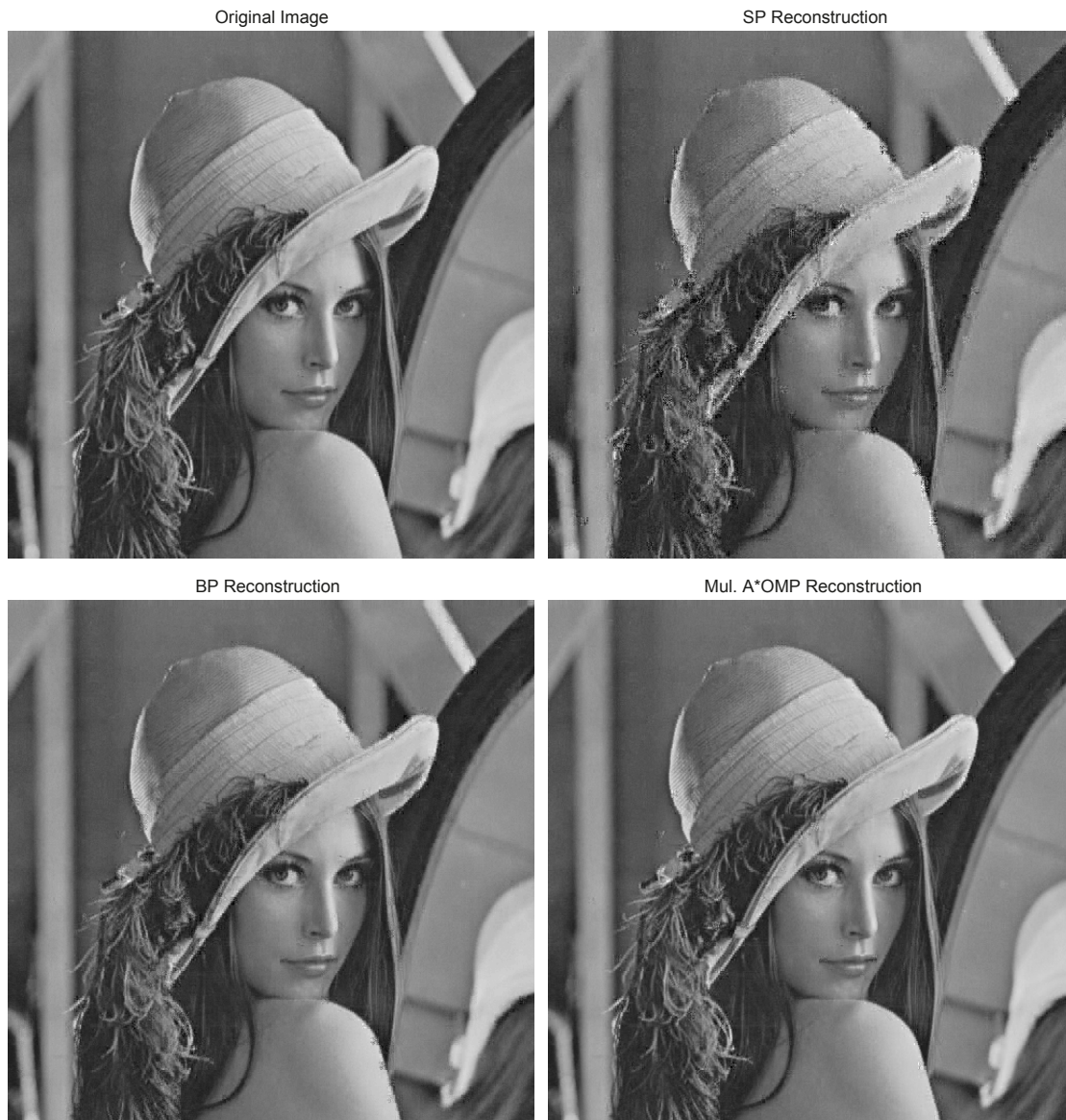
FIGURE 4.15: Reconstructions of the image “Lena” using BP, SP, and Mul-A*OMP with B = 3
