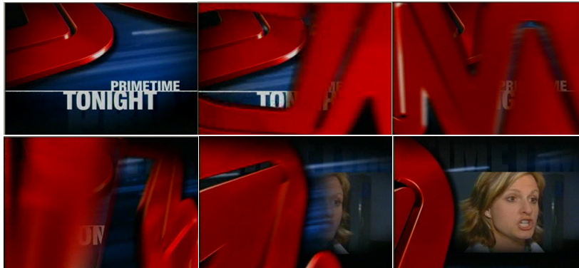
Figure 3.2 The CNN logo animation, frequently used between the shots in many test videos, is an example for the gradual transitions that can be detected by employing a dedicated transition detector.
