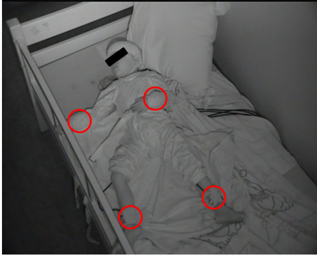
Figure 2.1: Acquisition setup the Pulderbos Rehabilitation Center for Children and Youth: the placements of wired accelerometers are indicated with red circles
