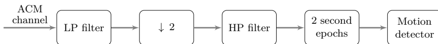
Figure 2.6: Schematic overview of preprocessing steps of ACM signals that result in motion epochs
