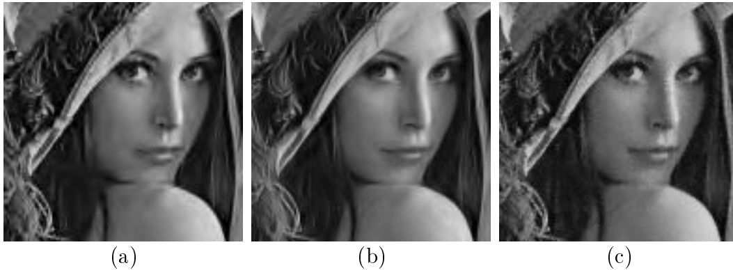
Figure 5.13: Lena after JPEG2000 compression (a), denoising (b) and denoising with remodulation attacks with 3 \times 3 window for estimating the watermark sign (c). Denoising attacks blur the image in a manner similar to compression, whereas the remodulated image looks noisier. The RMS error of the all images is about 6.3.
