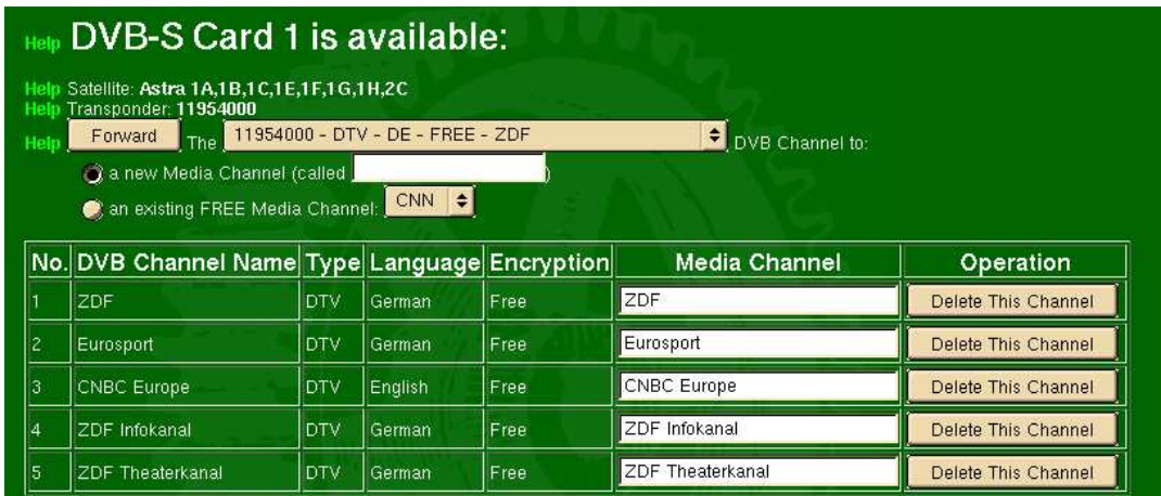
Figure 6.4: Screenshot of IP TV Server configuration: Assigning Channels to DVB-S Cards.
