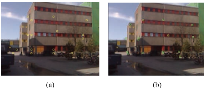
Fig 5. Feature selection: (a) using the sum of squared derivatives (b) using eigenvalue analysis.
