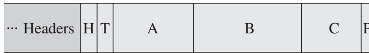
Figure 2.5: AMR RTP payload format: Bandwidth efficient mode [100]. Note that the H and T fields constitute the RTP payload header and are not part of the RTP header.
