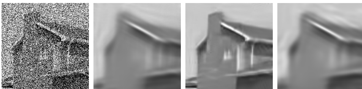
(e) Noisy image. Peak = 2. (f) NLSPCAbin. PSNR = 21.28dB. (g) BM3Dbin. PSNR = 24.23dB. (h) SPDAbin. PSNR = 21.39dB.
