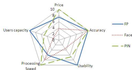
Figure 8.8: Comparison of fingerprint (FP), face recognition and PIN based access control systems.
