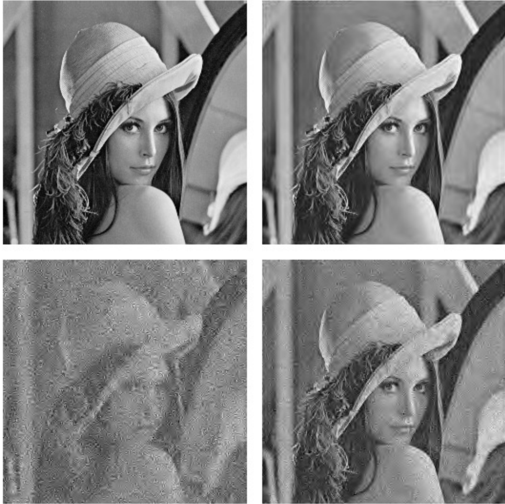
Figure 6.10: Top left: Original 256 \times 256 image. Top right: Best s -term approximation, s = 6000 , R-SNR=23.9 dB. Reconstruction from m = 16000 . Bottom left: LIHT, R-SNR=10.2 dB. Bottom right: LIHT-PKS k = 2000 , R-SNR=20.4 dB.
