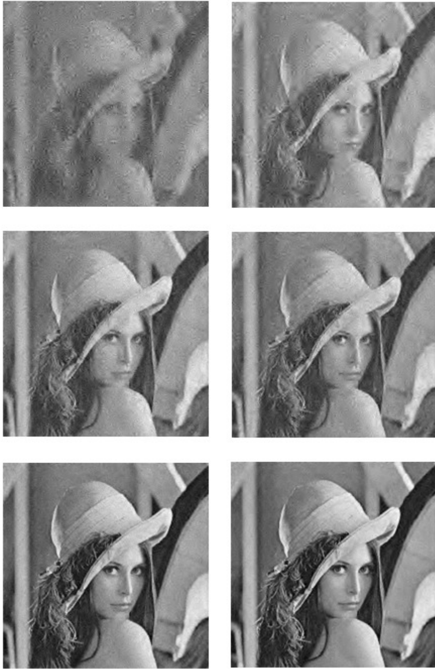
Figure 5.6: Image reconstruction example with Lena. Top row: m = 8000 . LBCS (left), PSNR=18.61 dB and GCBCS (right), PSNR=23.81 dB. Middle row: m = 20000 . LBCS (left), PSNR=25.56 dB and GCBCS (right), PSNR=26.36 dB. Bottom row m = 32000 . LBCS (left), PSNR=30.36 dB and GCBCS (right), PSNR=32.10 dB.
