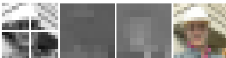
Fig 5. From left to right: Y, U and V components and reconstructed macroblock.
