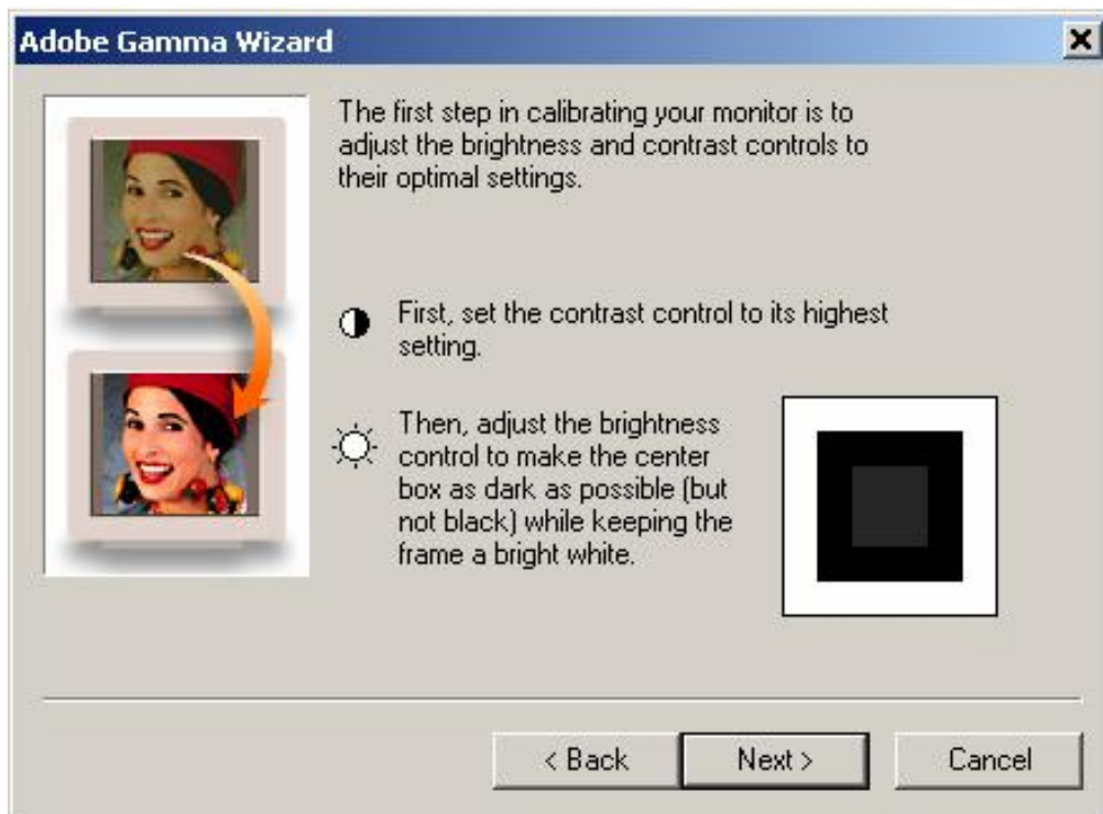
Figure 6.4. Adobe Gamma Wizard instruction dialogue box for optimal brightness and contrast settings.
