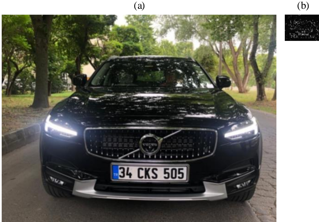
Figure 4.11 : Comparison of the size of the pixel domain image and the compressed domain image. a) A 1024 \times 768 pixel domain image. b) A compressed domain image corresponding to the pixel domain image with a resolution of 128 \times 96 pixels, where each CU is represented by a single pixel.
