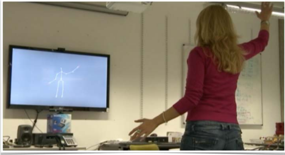
Figure 7.9: Kinect skeleton tracking controlling the prosody of pHTS. Left hand controls pitch and right hand the duration of the synthetic speech.
