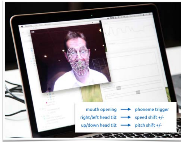
Figure 7.2: Reactive speech synthesis controlled by facial gestures. The head tilt controls prosody while the mouth opening triggers the RNLP module.
