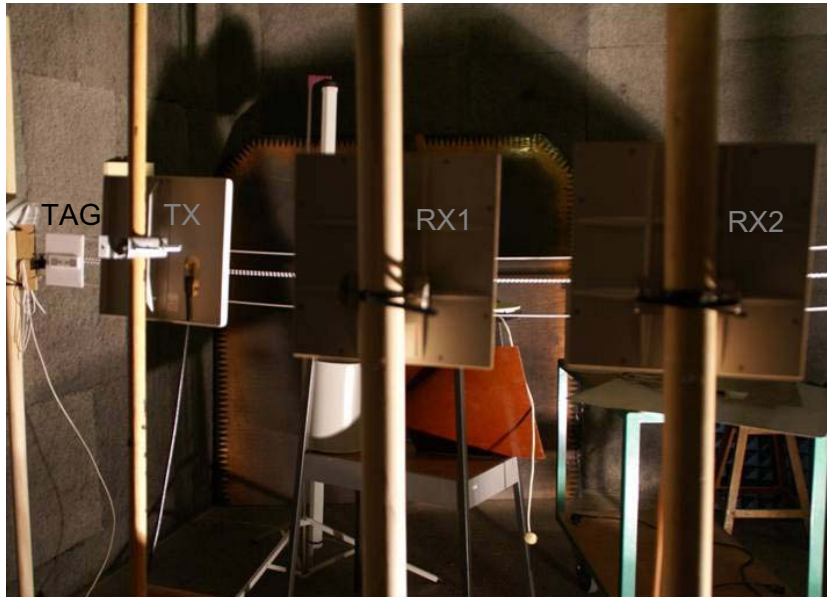
Figure 4.9: Measurement setup with TX (left) and RX (right) antennas. The tag is moved on the motor driven nylon cord through the measurement room. The fading in the room is generated artificially by placing one dominant ( \approx 2.5 \text{ m}^2 ) reflector in back left corner (position x=0 \text{ m} , y=0 \text{ m} ) and several smaller reflectors in the measurement scenario.
