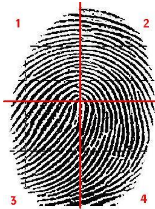
Figure 5-7 Block division of the fingerprint image
