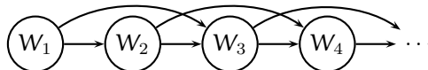
Figure 8.1 – A conceptual trigram dynamic Bayesian network. Every time slice contains a random variable W that takes the words in the vocabulary as its states.
