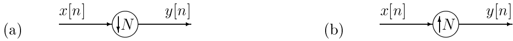
Figure 3.2: Basic multirate operations for sampling rate alteration: (a) decimation; (b) expansion of signal x[n] by a factor of N .
