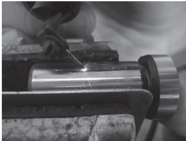
Figure 3.11: Localized inner ring defect being seeded.
