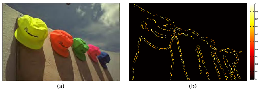
Fig. 14. Illustration of how the proposed NR ringing metric works on JPEG2000 compression: (a) a JPEG2000 coded image (bit rate 0.099 bpp) from LIVE database [43]; and (b) extracted visible ringing pixels with their visibility indicated with a color ranging from black (no visibility) to yellow for the highest visibility.
