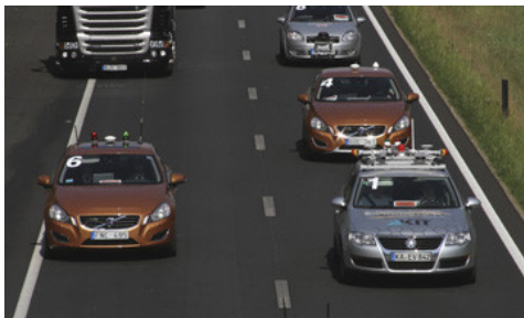
(a) Inertial sensors are used in combination with the global positioning system (GPS) to estimate the position of the cars in a challenge on cooperative and autonomous driving.
