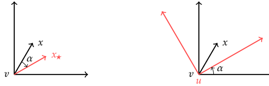
Figure 14: Left: clockwise rotation \alpha of the vector x to the vector x_\star . Right: counterclockwise rotation \alpha of the coordinate frame v to the coordinate frame u .
