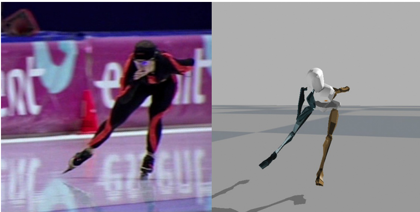
Figure 1: Example of inertial motion capture. Left: olympic and world champion speed skating Ireen Wüst wearing an inertial motion capture suit with 17 inertial sensors. Right: graphical representation of the estimated position and orientation of the body segments.
