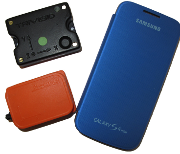
(a) Left bottom: an Xsens MTx IMU (Xsens Technologies B.V., 2016). Left top: a Trivision Colibri Wireless IMU (Trivision Prototyping GmbH, 2016). Right: a Samsung Galaxy S4 mini smartphone.
