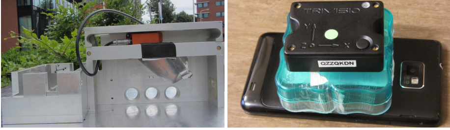
Figure 2: Left: experimental setup where a calibration experiment is performed outdoors. An Xsens MTi-100 IMU (orange box) together with a magnetic disturbance is placed in an aluminum block. Right: experimental setup using a Trivisio Colibri Wireless IMU (black box). A phone is used as a source of magnetic disturbance. To avoid saturation of the magnetometer, the phone is not attached directly to the IMU.
