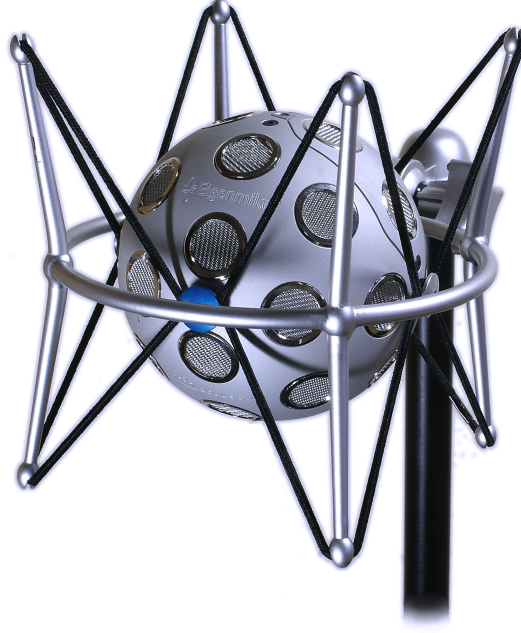
Figure 2.5: The em32 Eigenmike spherical microphone array. This rigid array of radius 4.2 cm is comprised of 32 omnidirectional microphones. (Photo credit: EMANUËL HABETS)
