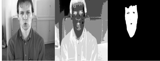
Figure 4.5: Test result of face segmentation in gray scale. The figure shows: (left to right) Delaunay Triangulation generated from points of the histogram, original image, Voronoi based image segmentation and segmented face, respectively.
