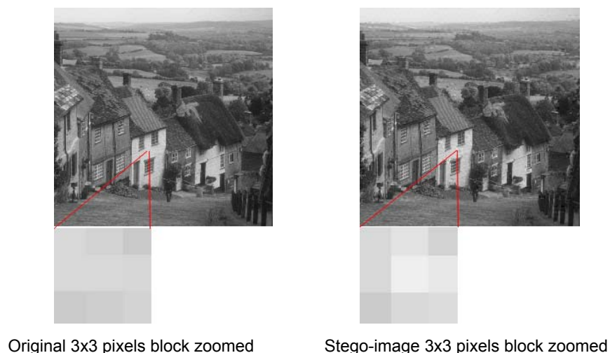
Figure 2.18: DCT embedding artefacts. (Left) patch from an original image (right) patch from the stego-image
