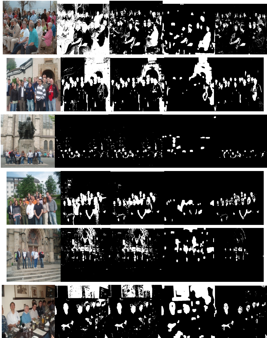
Figure 6.17: Performance analysis of skin tone detection on arbitrary images. (Left column to right) Original image, (Hsu et al., 2002) method, (Berens & Finlayson, 2000) method, (Kovač et al., 2003) method and the proposed method, respectively
