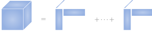
Figure 2.3: The more general block terms in a decomposition in multilinear rank- (L_r, L_r, 1) terms allow us to model more complex phenomena than what is possible with the simple rank-1 terms of the canonical polyadic decomposition.
