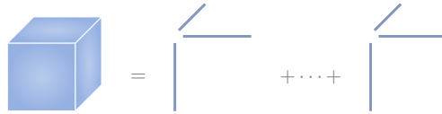
Figure 2.2: The polyadic decomposition writes a tensor as a sum of rank-1 terms and is a fundamental tool for signal separation because it is unique under fairly mild conditions.
