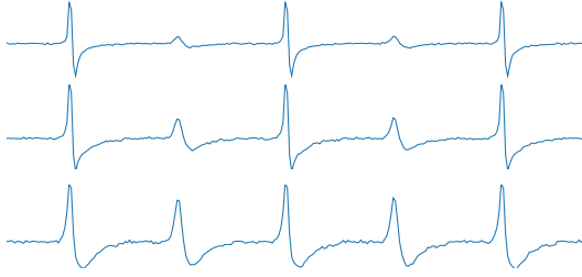
Figure 6.16: Simulated outputs of a high-density microelectrode array for measuring neuronal activity using simulated spike trains as inputs.
