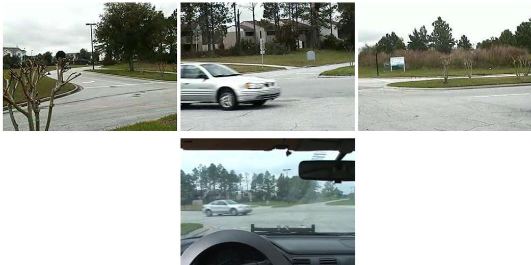
**Figure 5.8** The car has exited the view of the left camera, although it is still visible in the video from the camcorder. The computer vision system is turned off because it will now be the UGV's turn to cross the intersection.
