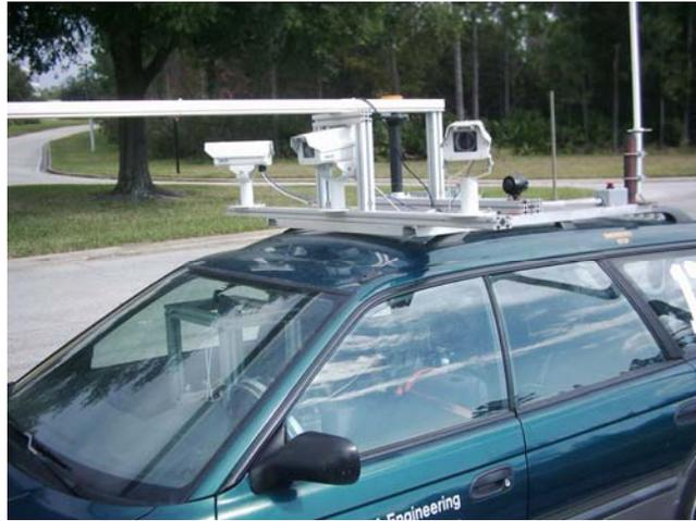
**Figure 5.2** The experimental UGV is a Subaru Outback with an autopilot system and three cameras mounted to the roof.
