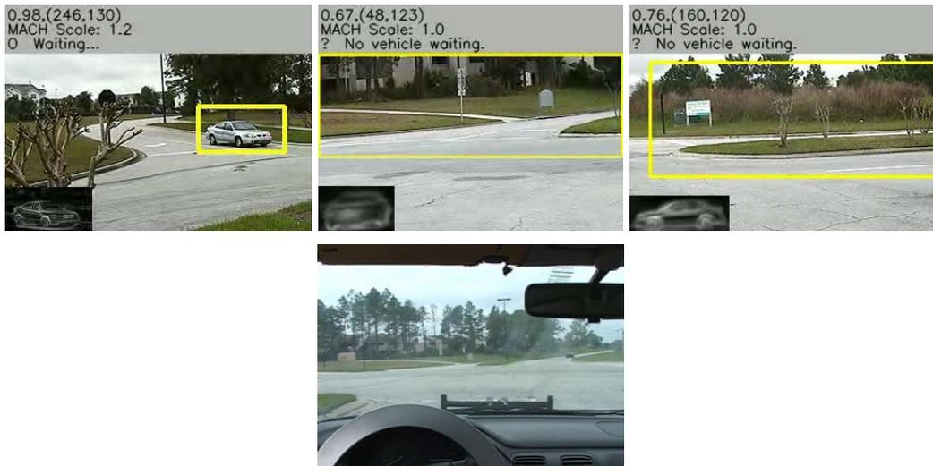
**Figure 5.6** The UGV stops and turns on the computer vision system. The system detects that the car is at the intersection and commands the UGV to wait.
