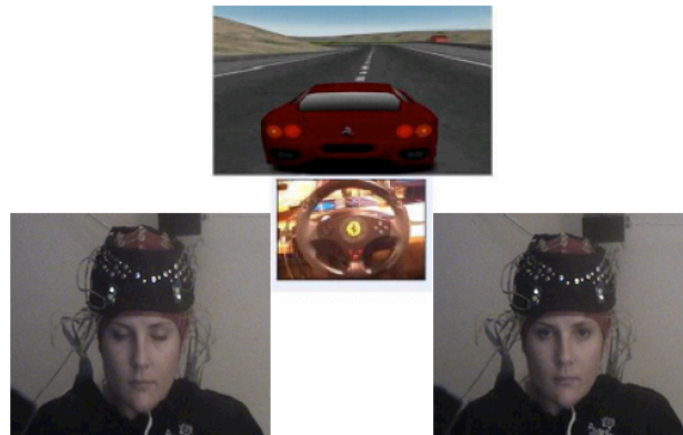
Figure 4.1: In this task samples of real sleep episodes were collected from 11 subjects while they were performing a driving simulator task at midnight for an entire 3 hour session.
