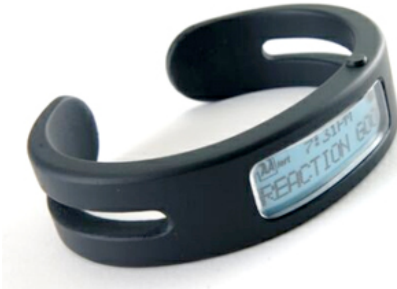
Figure 2.1: AAlert wristband driver drowsiness detection device developed by Dan Ruffle. The device uses motion combined with reaction time to determine whether or not the driver is in a drowsy state.
