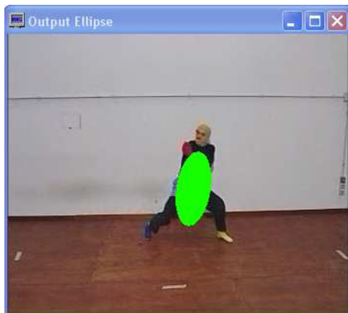
Figure 6.6: computation of an ellipse approximating the dancer's silhouette. The axes of the ellipse allow estimating the orientation of the body; its eccentricity is related to body contraction/expansion
