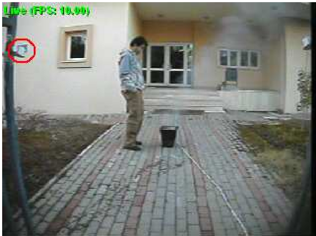
Figure 5.7: The PIR sensor is encircled. The fire is close to die out completely. A man is also within the viewing range of the sensor.
