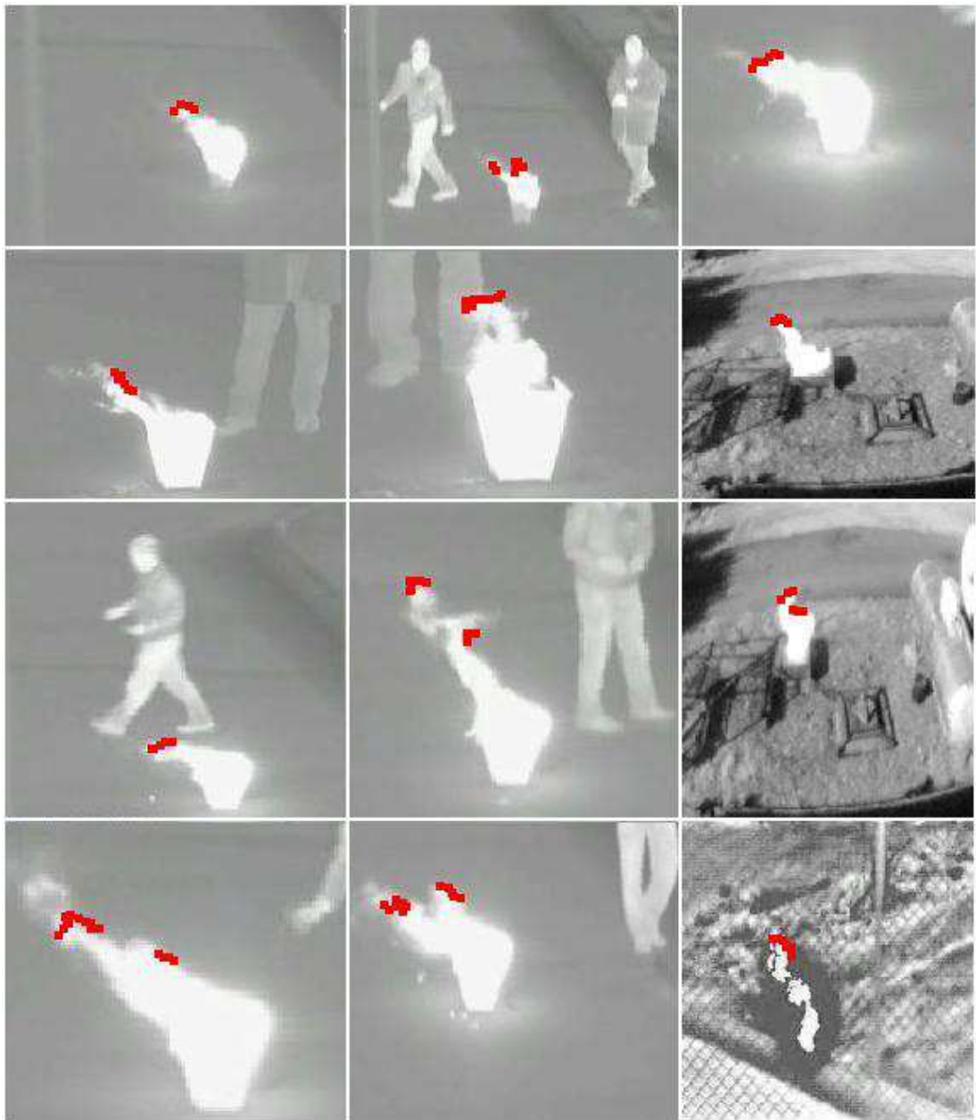
Figure 3.9: Image frames from some of the test clips with fire. Pixels on the flame boundaries are successfully detected.
