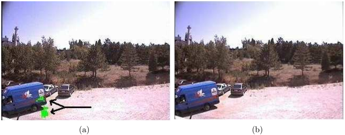
Figure 2.9: (a) With the method using color and temporal variation only (Method-2.2) [64], false alarms are issued for the fire colored line on the moving truck and the ground, (b) our method (Method-2.1) does not produce any false alarms.
