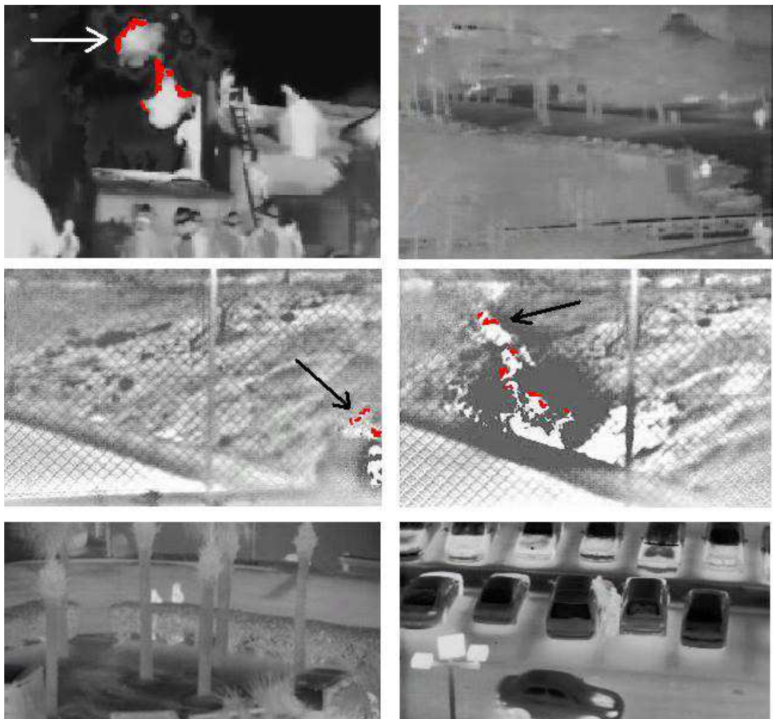
Figure 3.8: Image frames from some of the test clips. a), b) and c) Fire regions are detected and flame boundaries are marked with arrows. d), e) and f) No false alarms are issued for ordinary moving bright objects.
