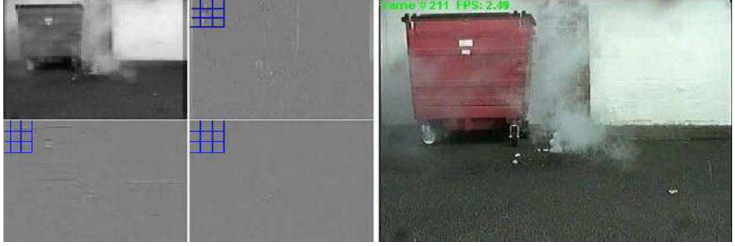
Figure 4.1: Image frame with smoke and its single level wavelet sub-images. Blurring in the edges is visible. The analysis is carried out in small blocks.
