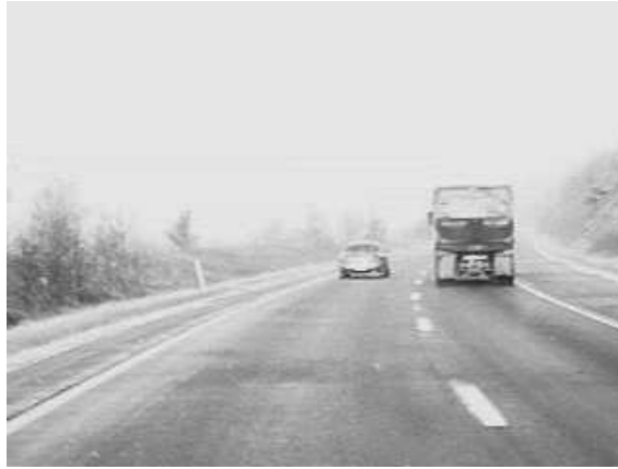
Figure 1.2: When entering a curve, all vehicles start moving in the lateral direction. This information can be used to support the road geometry estimate.
