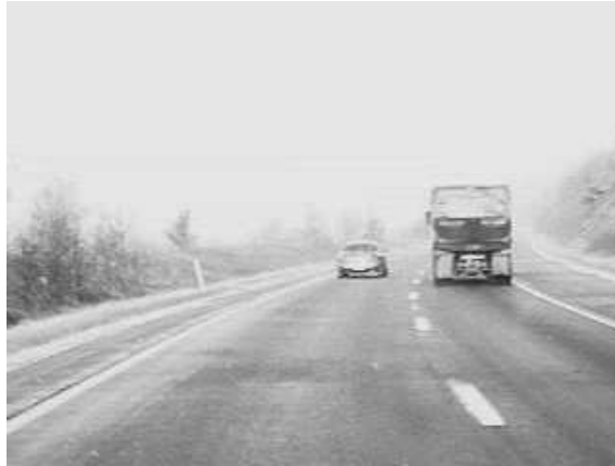
Figure 1: When entering a curve, all vehicles start moving in the lateral direction. This information can be used to support the road geometry estimate.
