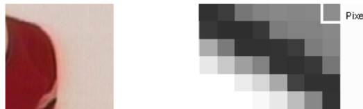
Figure 1.10: a) Colour bleeding b) Slanted lines.
