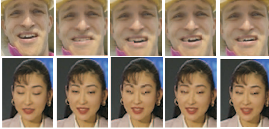
Figure 3.18: Screenshots of the video sequences “foreman” (upper row) and “akiyo” (lower row): correctly received previous ROI \underline{R}_{n-1} , original ROI \underline{R}_n , reconstructions by copy-paste, boundary matching, and block matching with 8 \times 8 blocks.
