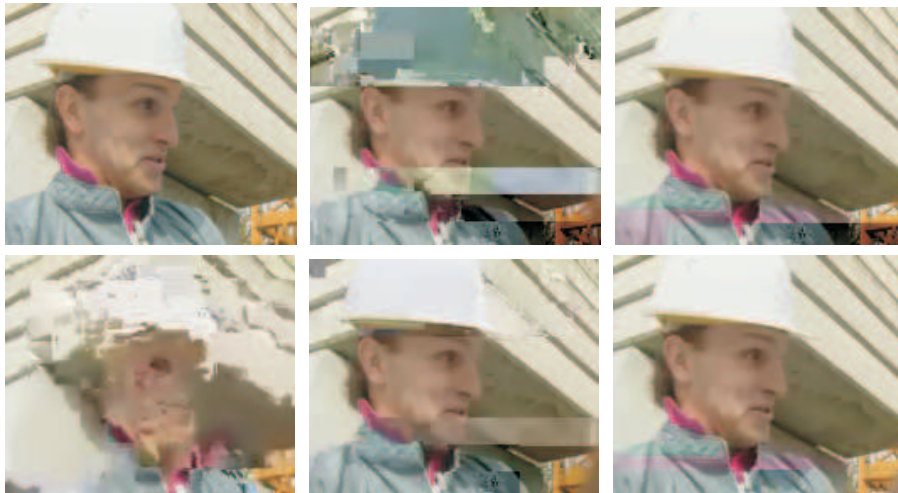
Figure 2.28: Screenshots from the “foreman”: original and concealed packet loss (left); sequential decoding without and with postprocessing (middle); sequential decoding with resynchronization, without and with postprocessing (right).
