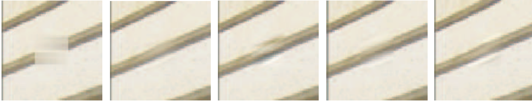
Figure 3.14: Quality of reconstruction after 100 iterations (from left to right): weighted averaging as initial guess POCS R = 7 and B = 3 with Tukey window, POCS R = 7 and B = 7 with rectangular window, POCS R = 5 and B = 2 with Tukey window, POCS R = 5 and B = 2 with rectangular window.
