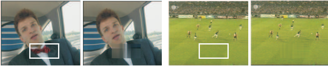
Figure 3.3: Performance of weighted averaging: concealment of a missing part in “carphone” and in “soccer” video picture. White rectangle marks the area to be concealed.
