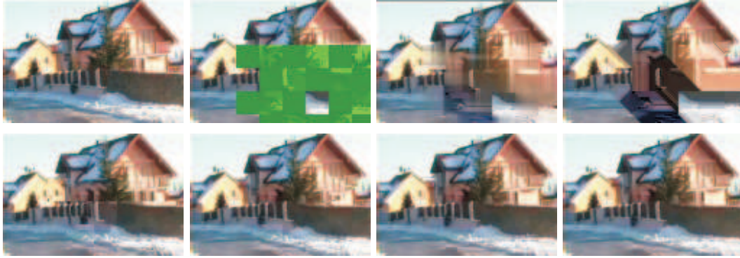
Figure 3.25: Screenshots of a part of an I frame in the “panorama” sequence: compressed original (Y-PSNR= 35.86 dB), error pattern (Y-PSNR= 10.45 dB), weighted averaging (Y-PSNR= 18.09 dB), directional interpolation (Y-PSNR= 16.57 dB), copy-paste (Y-PSNR= 22.76 dB), boundary matching (Y-PSNR= 26.27 dB), 8 \times 8 block matching with (Y-PSNR= 30.27 dB), 2 \times 2 block matching with (Y-PSNR= 30.74 dB).
