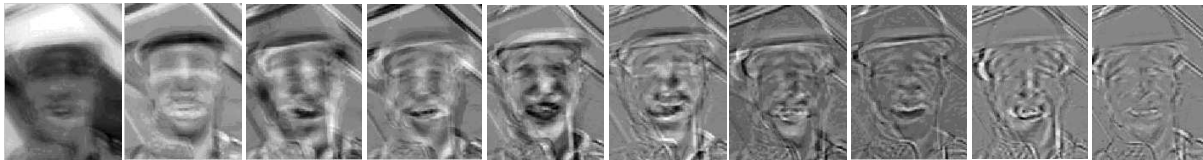
Figure 3.19: Mean image \underline{M} and eigenfaces \underline{U}_k obtained from 10 successive luminance ROI images of the sequence ‘foreman’.
