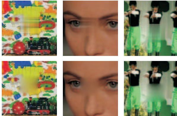
Figure 3.8: Images reconstructed by weighted averaging (upper row) and smoothing (lower row).
