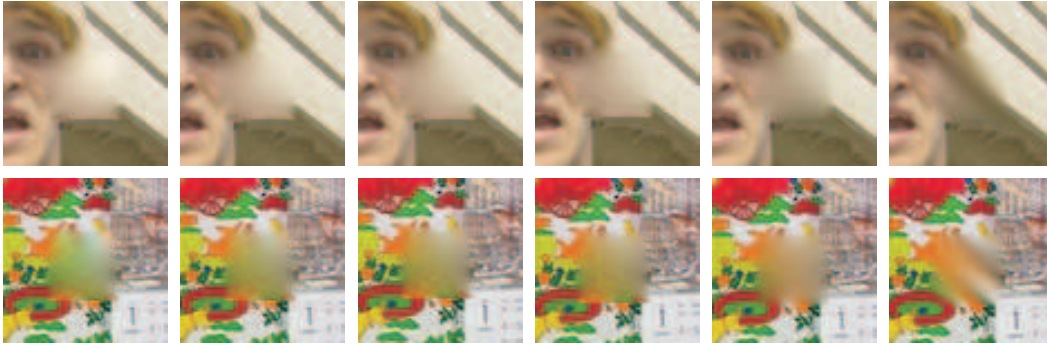
Figure 3.10: Images reconstructed by second order derivative smoothing with (left to right) \lambda = 0, 1, 2, 4 and by the first order derivative smoothing without and with edge awareness.
