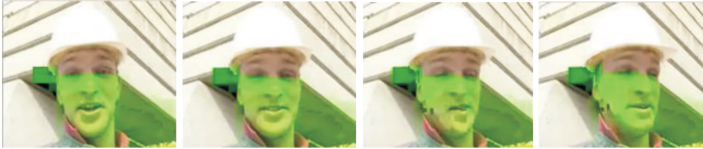
Figure 1.5: Example of the spatial and temporal error propagation in a H.264/AVC encoded video sequence “foreman”.
