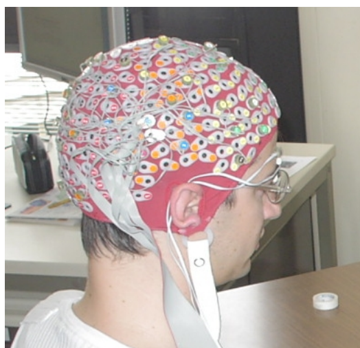
Figure 3.2. (left) A participant wearing the EEG cap with 64 electrodes plugged. (right) Top head view with the positions and names of the 64 electrodes used for EEG recording. For a 19 electrodes configuration only the green electrodes were used.
